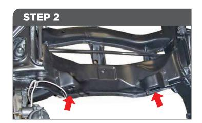
Undo the two nuts on the lower control arm bolts, if your nuts are facing the other side you will need to install the lower control arm bolts with the nuts facing towards the firewall (This is standard)
