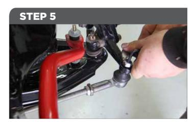
Using an allen key and a spanner tighten up the locking nut on the tie rod ends.
