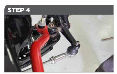
Install the steering arms that come with the kit onto the spindles. Install the Tie Rod ends on the rack and connect to the steering arms.
