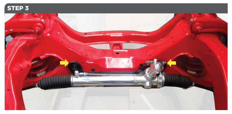
Lift the RetroRack Rack that is mounted to the Black bracket onto the lower control arm bolts as shown in the above photo.
