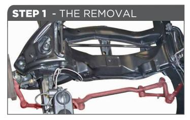
Remove the original steering components such as the steering box, drag link, idler arm, tie rod ends and the steering arms.
