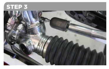
Install the steering arms without the rubber boots to the Rack and pinions draglink by screwing it on, install both arms one on each side of the drag link.
