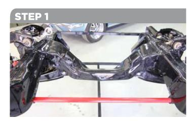
Remove the original steering components such as the steering box, drag link, idler arm and tie rod ends. The RetroRack Bolt in Kit utilises the original mounting points in your chassis.
