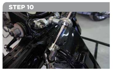
Install the support bearing bracket to the upper control arm. Connect to steering shaft, additional universal joint, and steering column depending on your application.
