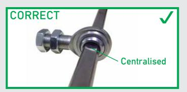
Make sure the Support bearing is not binding on the steering shaft. The support bearing nuts should not be done up so the support bearing is pulling on the shaft, the shaft should be centralised in all directions.
