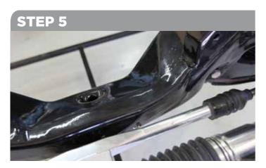
Install the lubricated rubber boots over the steering arms.
