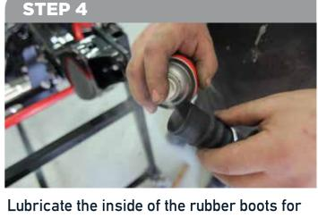
the steering arms using WD40 or similar. This is required to prevent rubber tearing if removal is required for wheel alignment.
