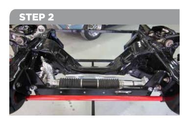
Lift the RetroRack Rack that is mounted to the Black bracket into place and insert the bracket bolts from the kit into the original steering mounting holes in your chassis.
